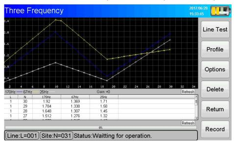
Using the three frequency and forming the curve like above, then find out the abnormal point of high value or low value; Choose the **high value of point 10 or lower value of point 19** to make the profile survey measurement.
